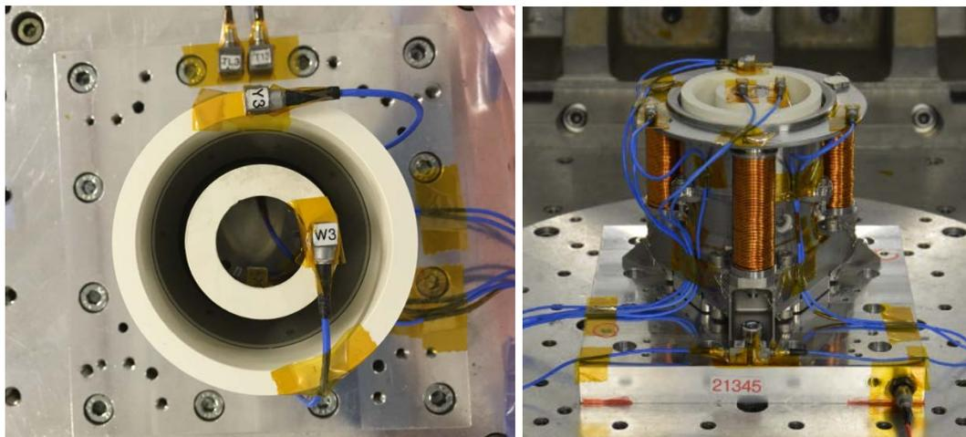
Figure 6. The PPS@X00 discharge chamber (left) and thruster structural model (right) during mechanical tests.
