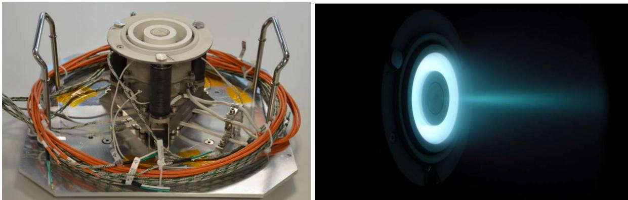
Figure 5. The first engineering model of the PPS®X00. Left: after manufacturing. Right: During firing in the PIVOINE-2g vacuum chamber.
