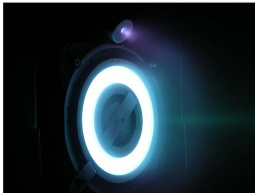
**Figure 3.** The PPS®1350-G DT firing with the PPS®X00 ceramic material.
