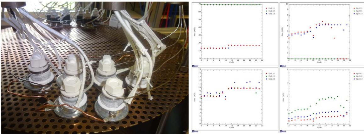
Figure 8. Coil thermal cycling test between  $-70^{\circ}\text{C}$  and  $+475^{\circ}\text{C}$ . Left: the two coil sample configurations on the thermal interface plate. Right: Insulation properties of the samples during the 25 first cycles.
