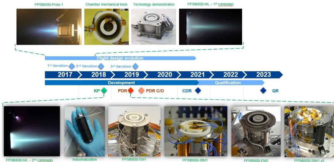
Figure 1. Illustration of the hardware that has been manufactured and tested during the preliminary design phase.
