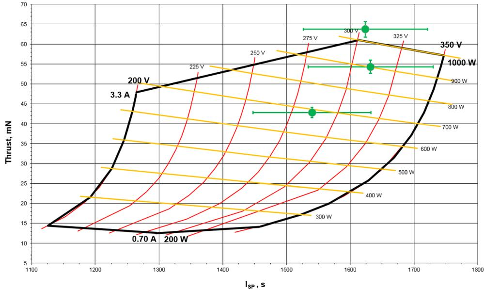
**Figure 2. PPS®X00 operating envelope. Green dots: performance measurements at 300 V and 650 W, 800 W and 1 kW.**
