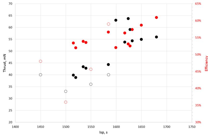
Figure 4. (Black) Thrust vs specific impulse. (Red) Efficiency vs specific impulse. Full symbols correspond to PPS®X00-ML performance measurements. Open symbols represent competitors performance extracted from the literature.
