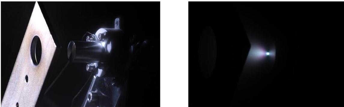
**Figure 11. Stand-alone test at SITAEL: HC3 mounted on the test setup (left) and operating with anode plate (right).**
