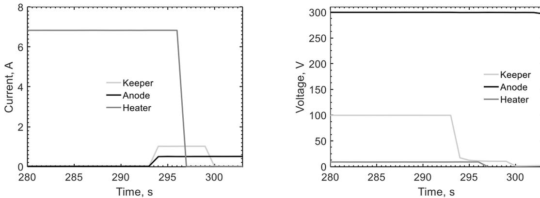
**Figure 7. Thruster ignition sequence at the end of the heating transient: currents (left) and voltages (right).**
