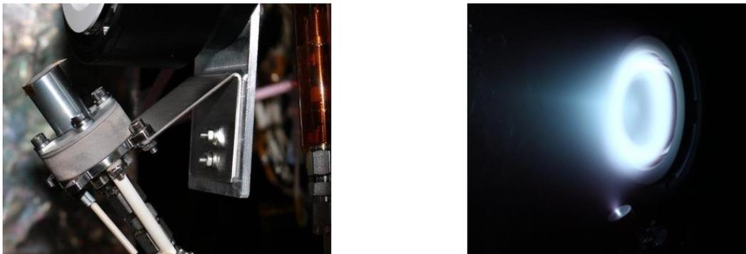
**Figure 13. Coupling test in IV4 (SITAEL): HC3 mounted on the test setup (left) and operating with MSHT400<sup>20</sup> (right).**
