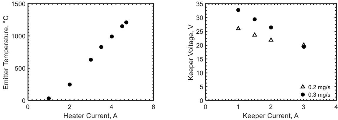
**Figure 10. Emitter temperature as a function of heater current (left), keeper voltage as a function of keeper current (right).**
