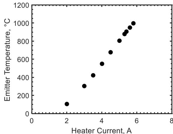
**Figure 5. Emitter temperature as a function of heater current.**
