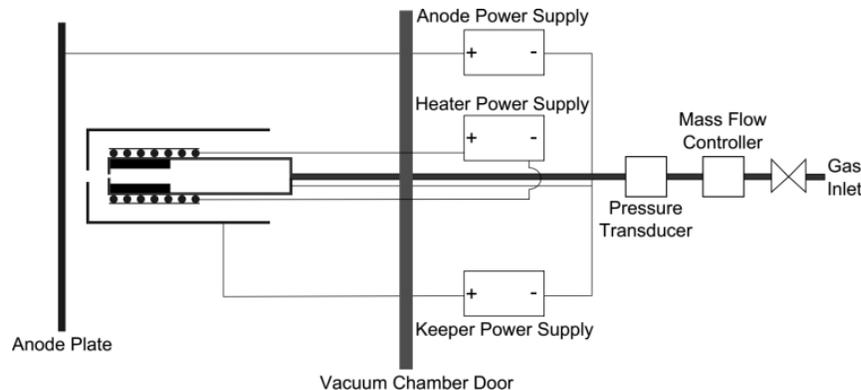
Figure 4. Setup schematic for HC3 stand-alone test.
