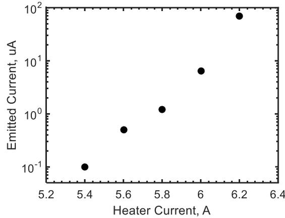
**Figure 6. Emitted current as a function of heater current.**
