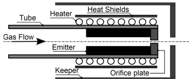
**Figure 1. General schematic of an orificed hollow cathode.**
