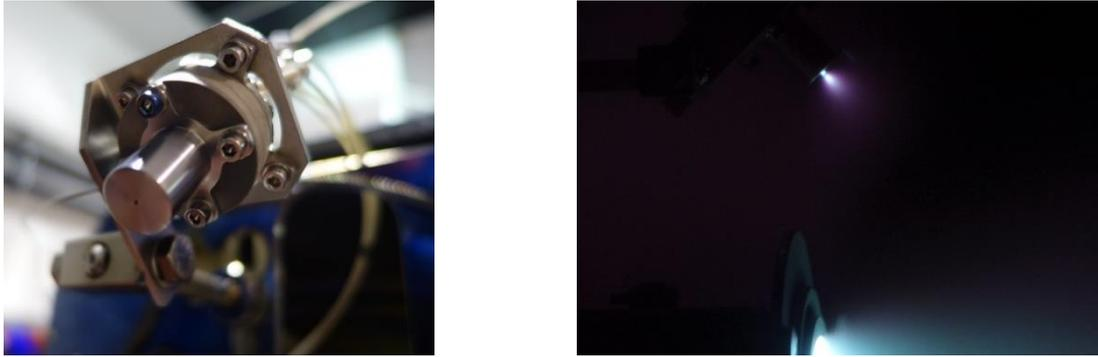
**Figure 12. Coupling test in PIVOINE (ICARE-CNRS): HC3 mounted on the test setup (left) and operating with Safran's PPS<sup>®</sup>X00<sup>19</sup>(right).**
