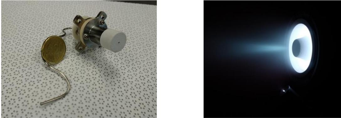
**Figure 8. HC1 assembled (left), and operating with HT100 (right).**
