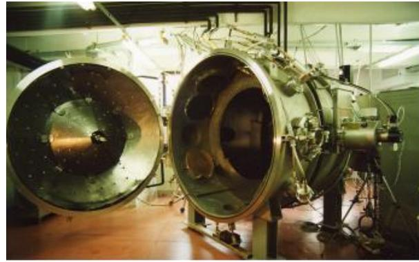
Figure 2. IV7 (left) and IV4 (right) vacuum chambers.
