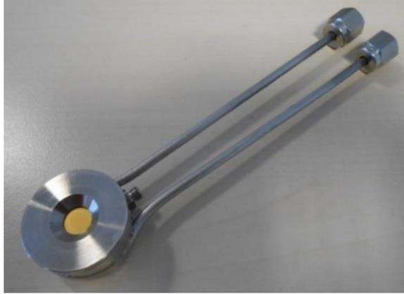
**Figure 9: QCM sensor during acceptance.**
