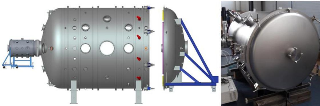
**Figure 8: IV10 rendering with the auxiliary chamber (left), auxiliary chamber during acceptance.**
