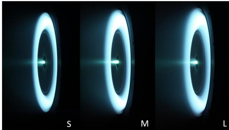
**Figure 7: HT20k DM2 firing at 300V and 25mg/s to the anode, from the S to the L configuration, first characterization campaign.**
