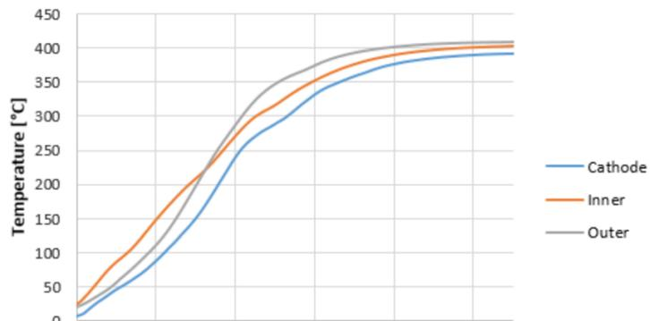
Figure 3: Thermal transient of the HT20k DM1 at 400V of discharge voltage and 20kW of discharge power.
