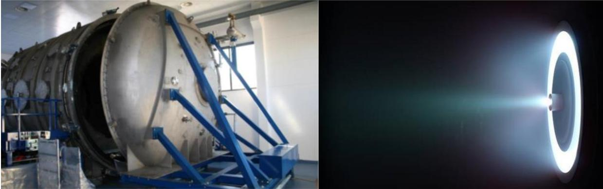
Figure 2: (left) SITAEL's IV10 space simulator. (right) HT20k-TU DM1, at 800 V and 20 kW of discharge power.
