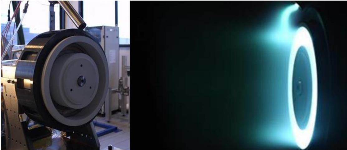
**Figure 4: HT20k-TU DM1 mounted on the thrust stand for the second campaign (left) and firing at 300 V and 15 kW with external cathode.**
