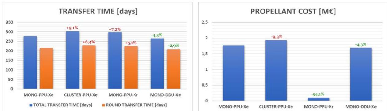
Figure 13: (left) total and round transfer time, (right) propellant cost estimation for the four investigated alternative architectures.
