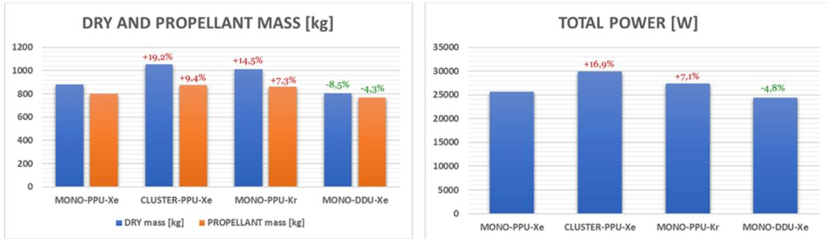
Figure 12: (left) dry and propellant budget, (right) power budget for the four investigated alternative architectures.
