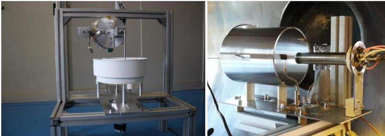
**Figure 5: Dedicated test setup to study the uniformity of the gas distribution (left), HC60 before the characterization test(right).**
